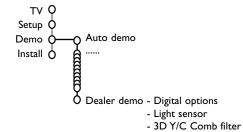
The Demo menu allows to demonstrate the TV features separately or in a continuous loop.
